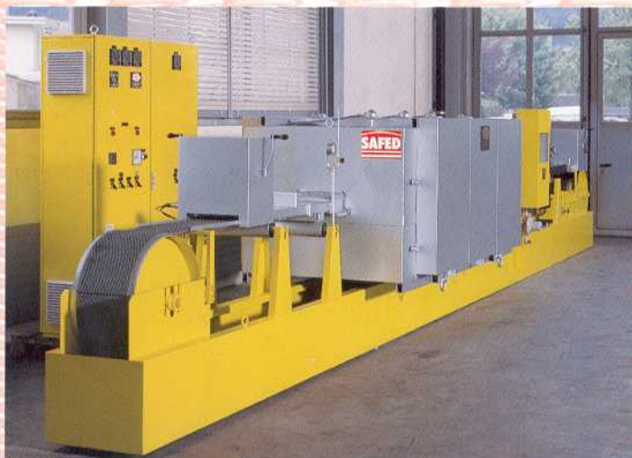
Furnace type 11 Bd 30/21 for hardening knife blades; electrically heated.
