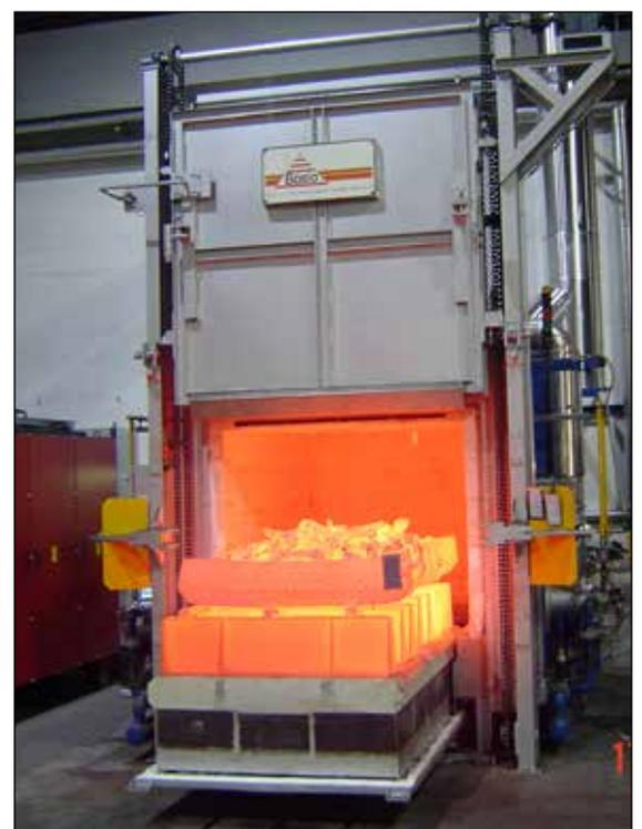
gas heated bogie hearth furnace - 3 m<sup>3</sup> - 1100°C
