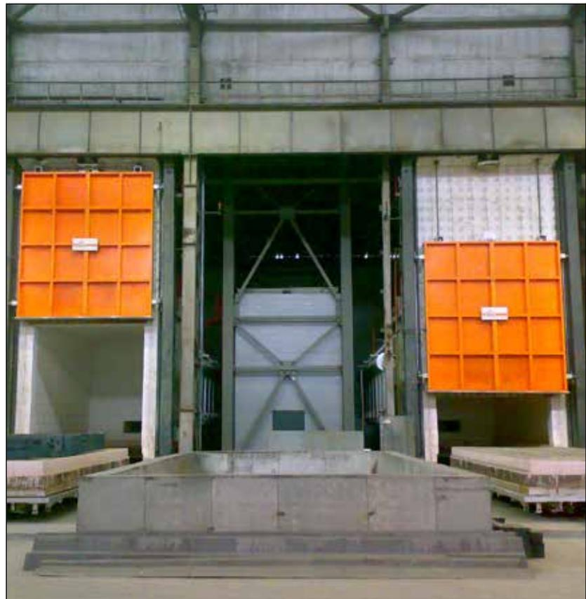
gas heated bogie hearth furnaces - 59 m<sup>3</sup> - 1200°C
