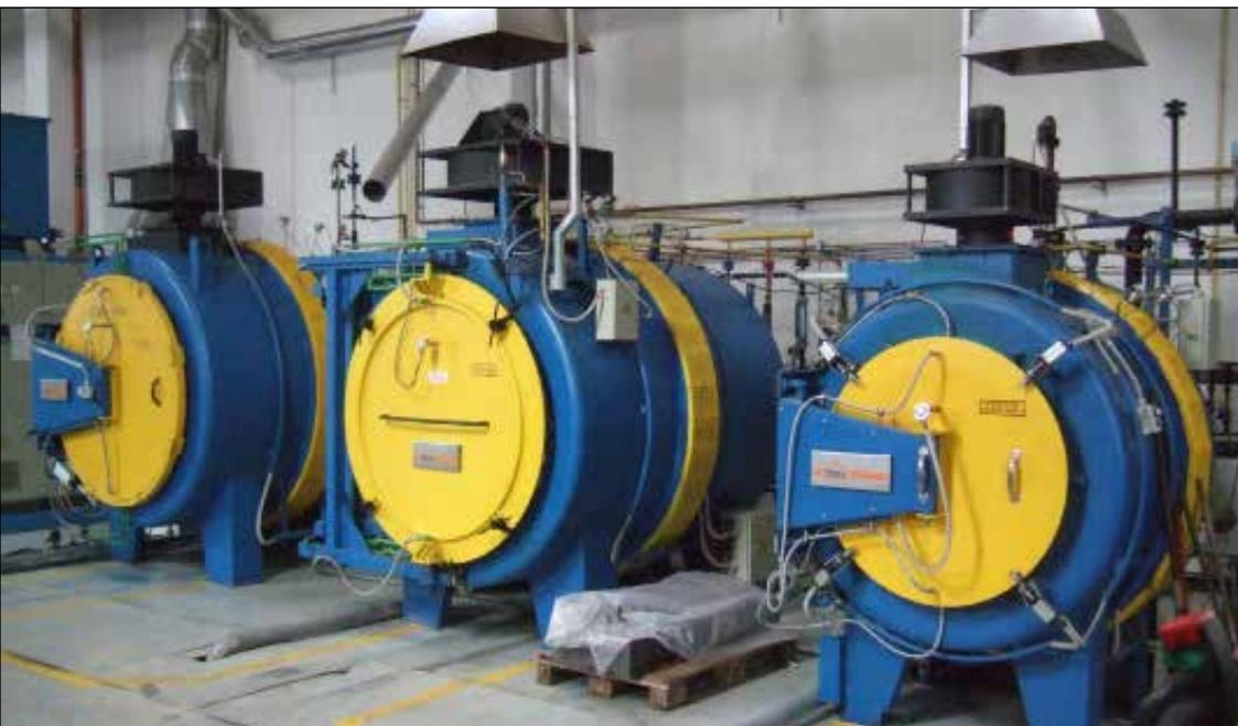
electro heated chamber furnace with rapid cooling (controled atmosphere)
