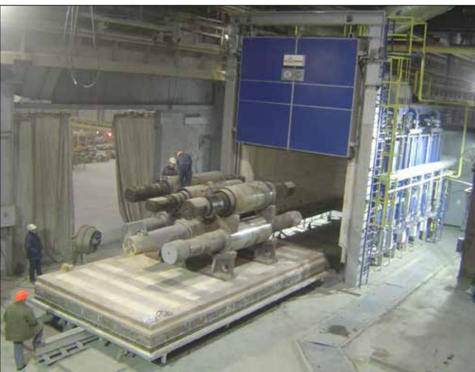
gas heated bogie hearth furnace - 70 m<sup>3</sup> - 1200°C
