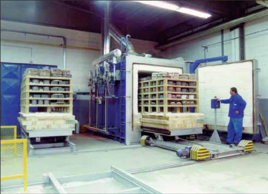
gas heated bogie hearth furnace - 5m<sup>3</sup> - 1300°C
