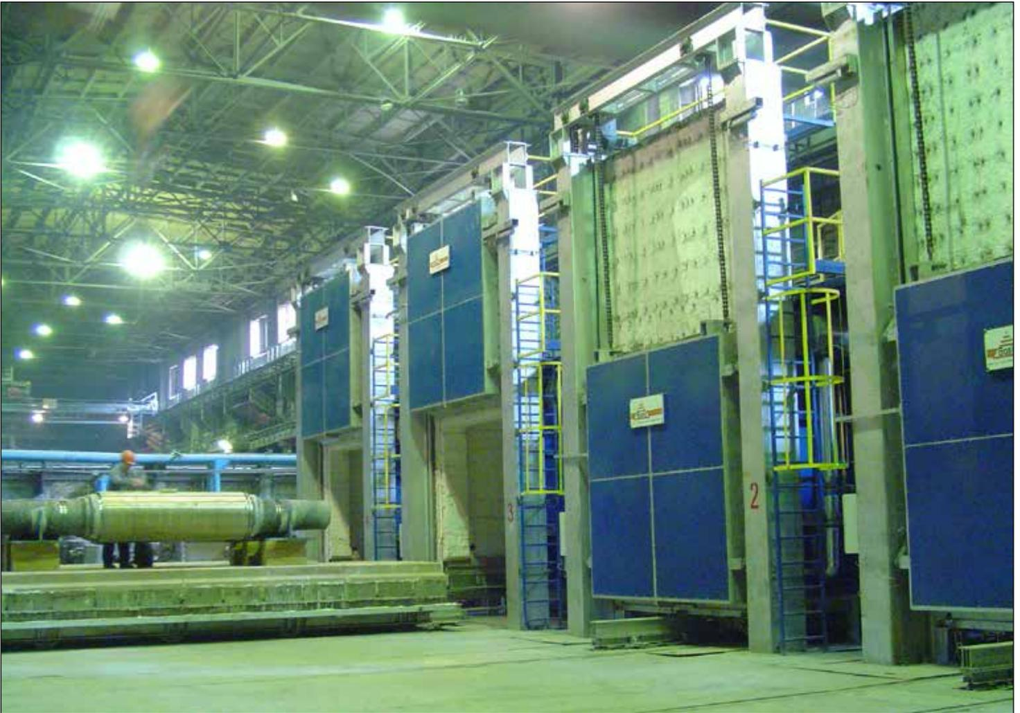
gas heated bogie hearth furnace - 34 m<sup>3</sup> - 1200°C
