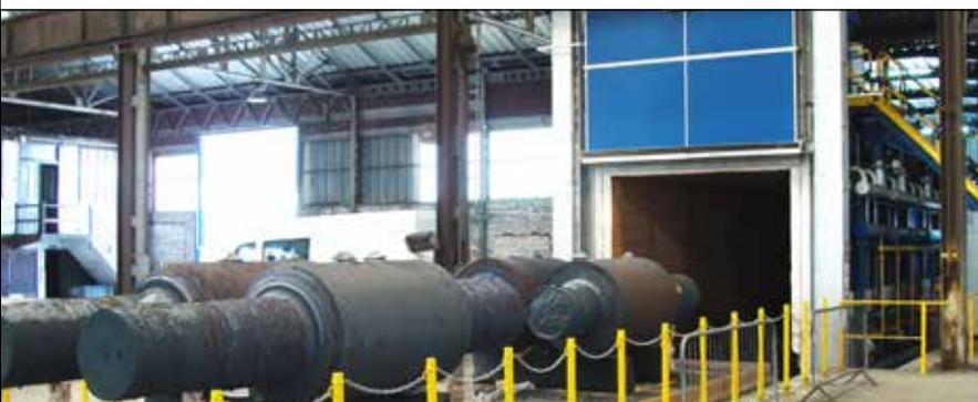
gas heated bogie hearth furnace -112 m<sup>3</sup>- 1150°C
