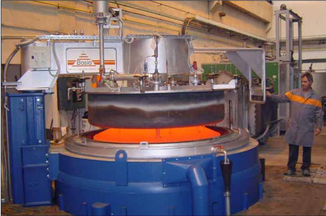
electro heated pit furnace (controled atmosphere) - 9 m<sup>3</sup> - 950°C
