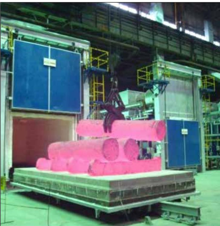
gas heated bogie hearth furnace - 47 m<sup>3</sup> - 1100°C
