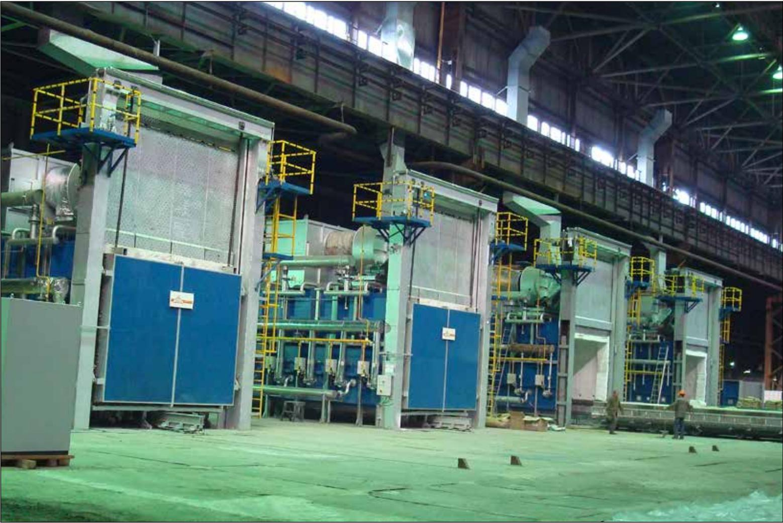
gas heated bogie hearth furnaces - 47 m<sup>3</sup>- 1100°C
