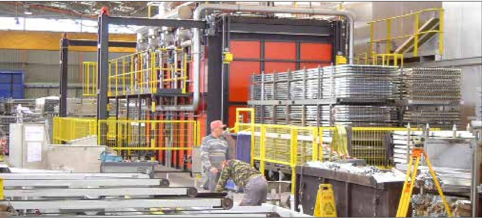
gas heated oven - 15 tons - 250°C
