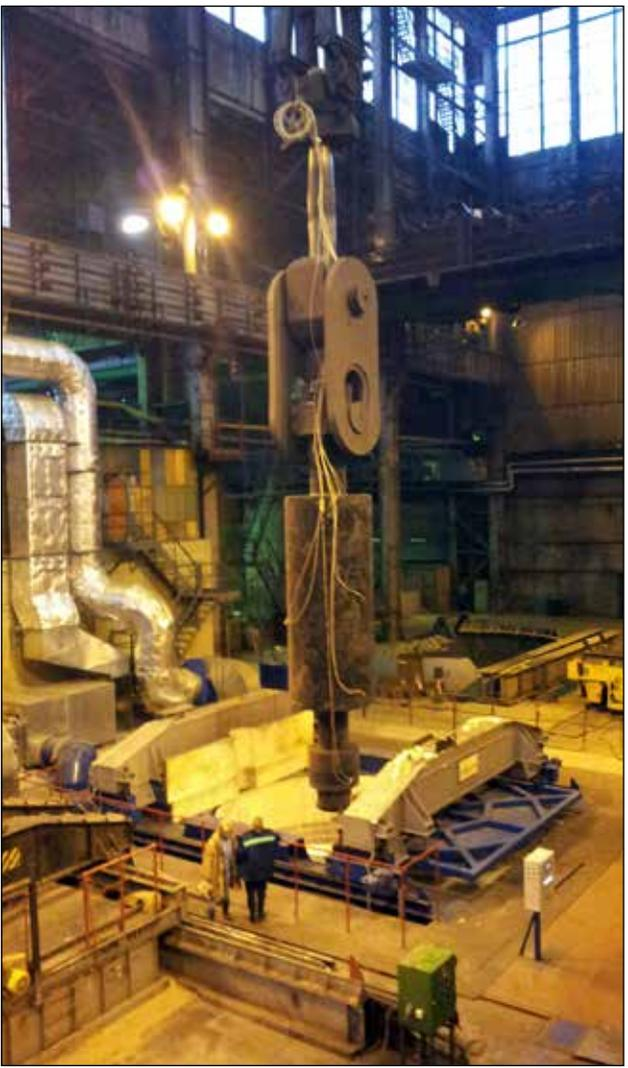
electro heated pit furnace - 175 tons - 22 m load height 1100°C
