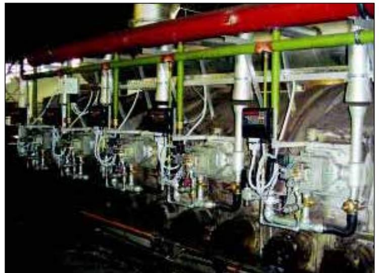
reconstructed gas heated tunnel furnace
