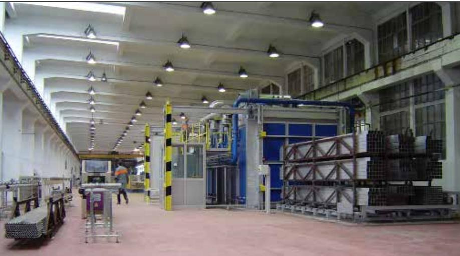
gas heated oven - 12 tons - 250°C
