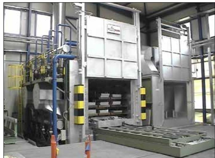
gas heated furnace and cooling chamber - 20 m<sup>3</sup> - 450°C
