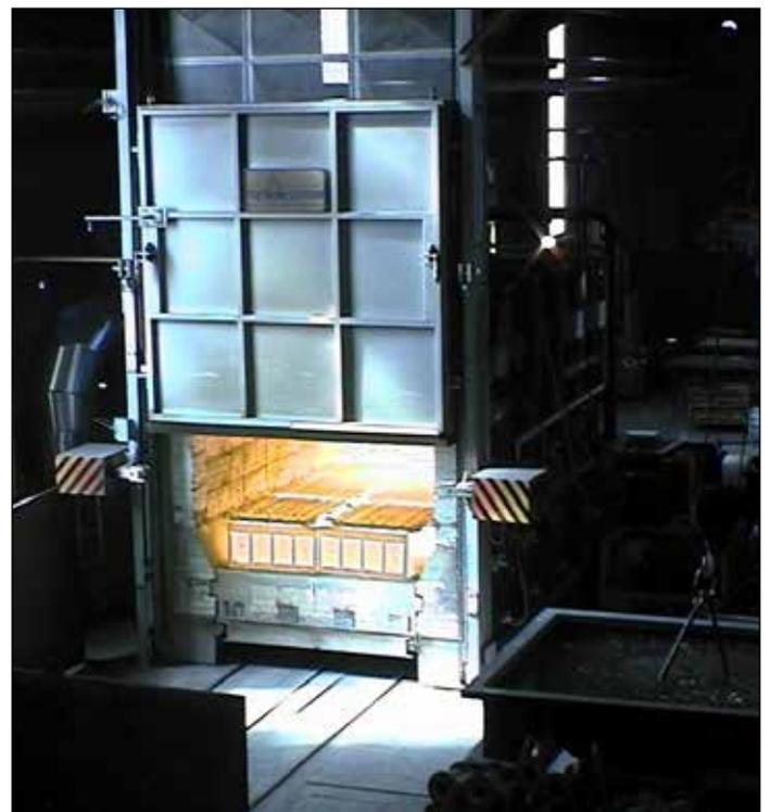
gas heated bogie hearth furnace - 12 m<sup>3</sup> - 1200°C
