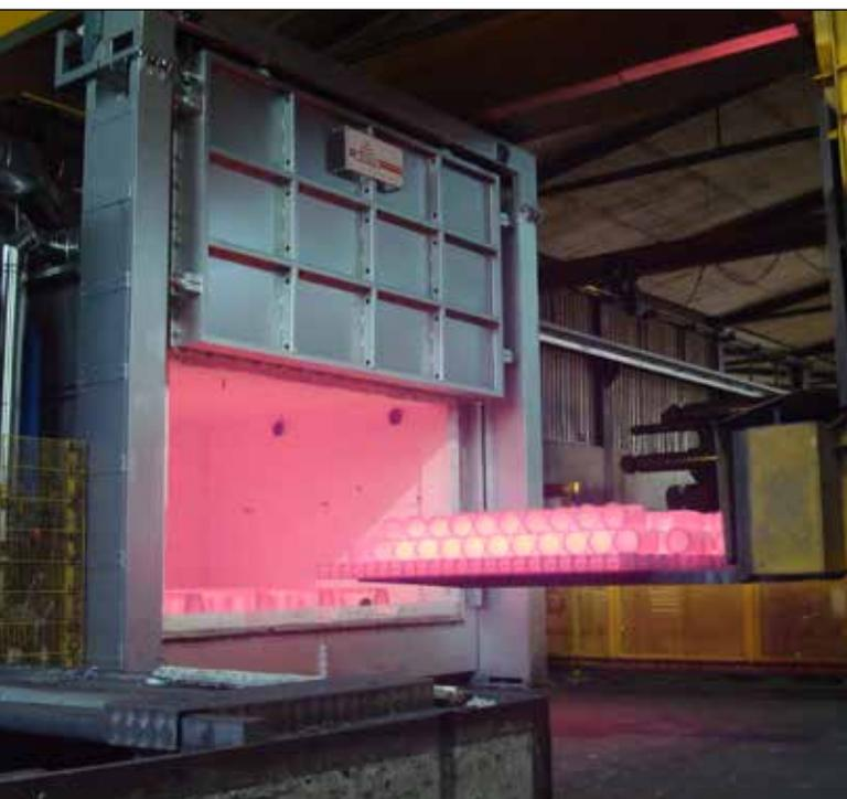
gas heated chamber furnace - 6m<sup>3</sup> - 1300°C
