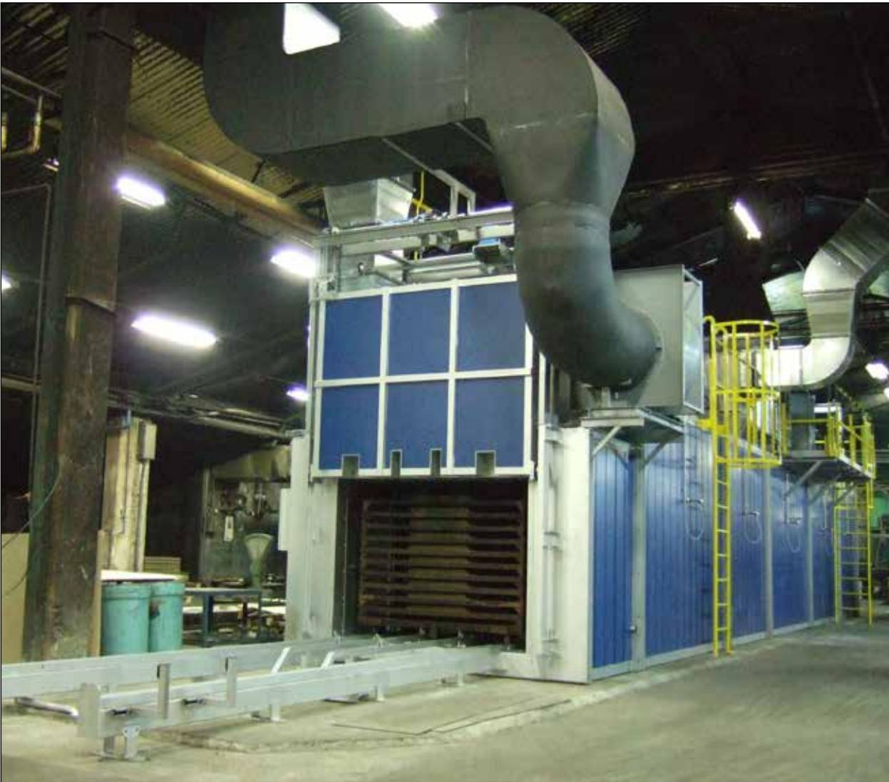
gas heated tunnel furnace
