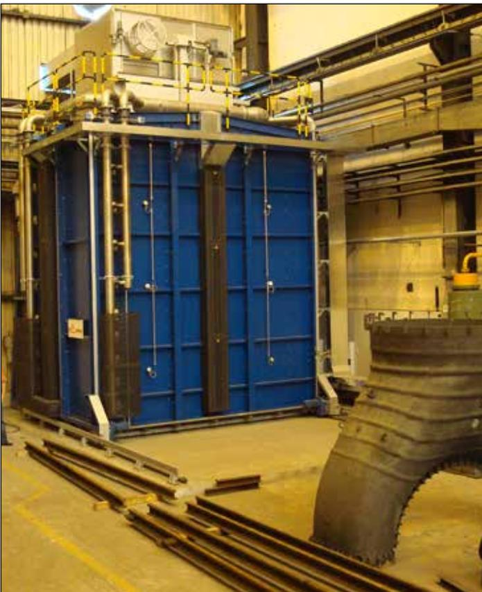
electro heated furnace - 56 m<sup>3</sup> - 1200°C
