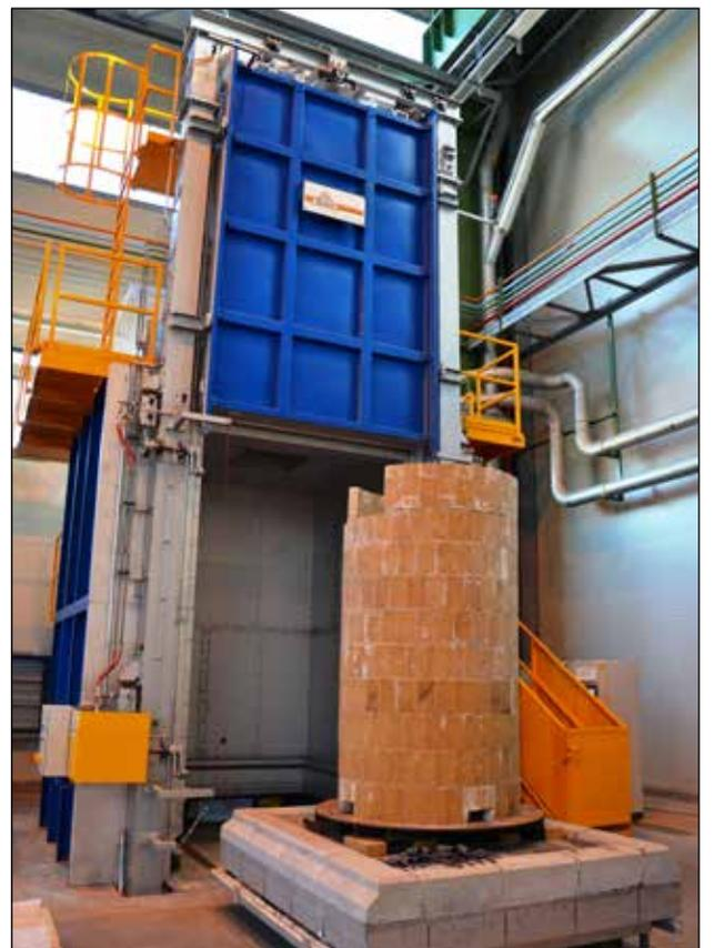
gas heated bogie hearth furnace - 12 m<sup>3</sup>- 300°C
