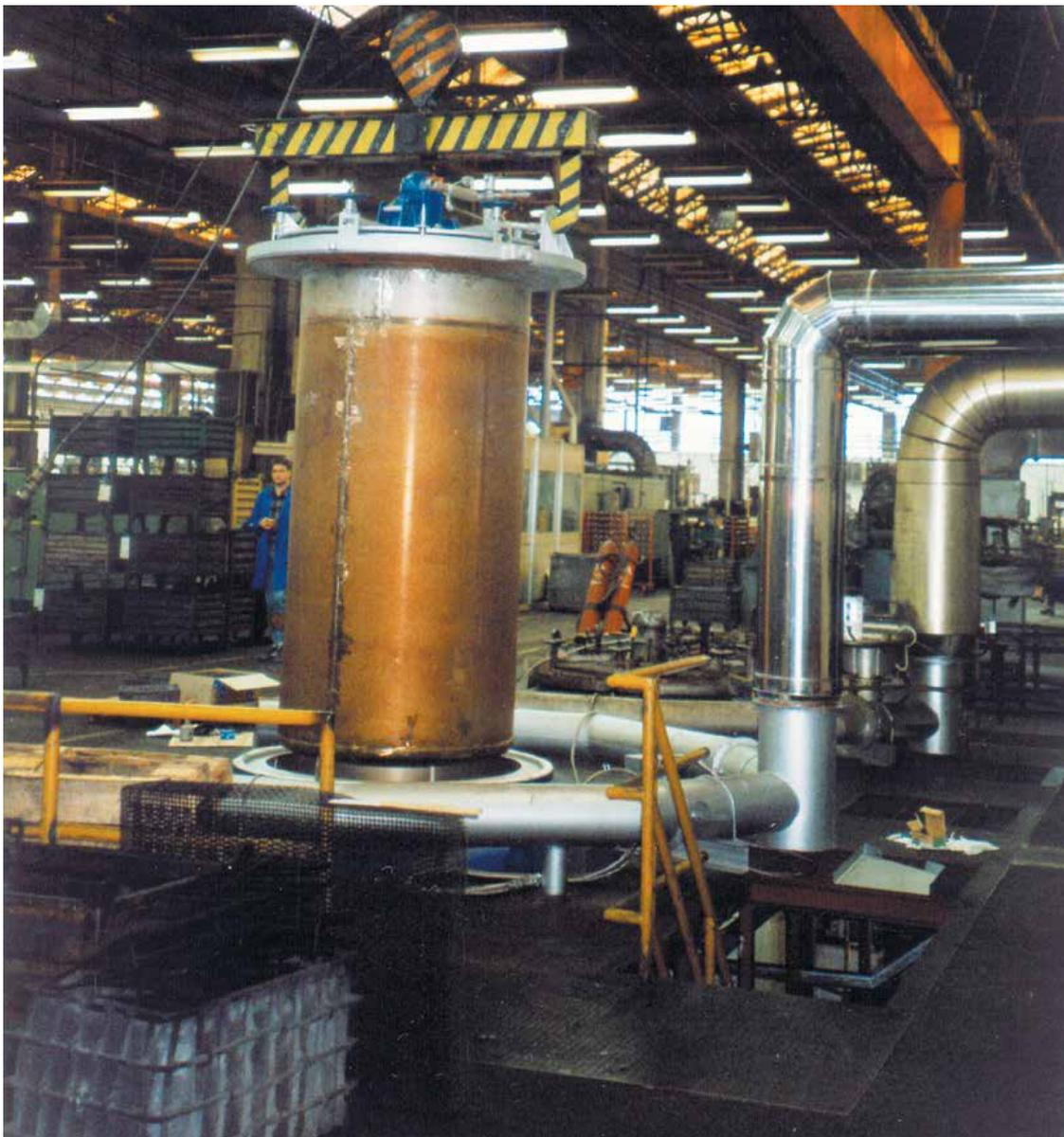
electro heated pit furnace (controled atmosphere)
