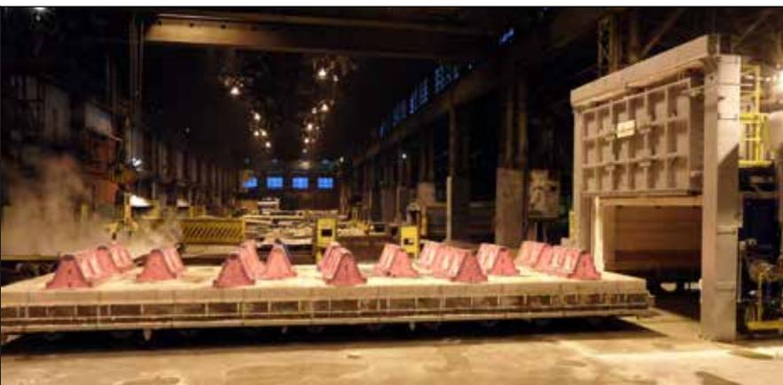
gas heated bogie hearth furnace – 51 m<sup>3</sup> – 1200°C
