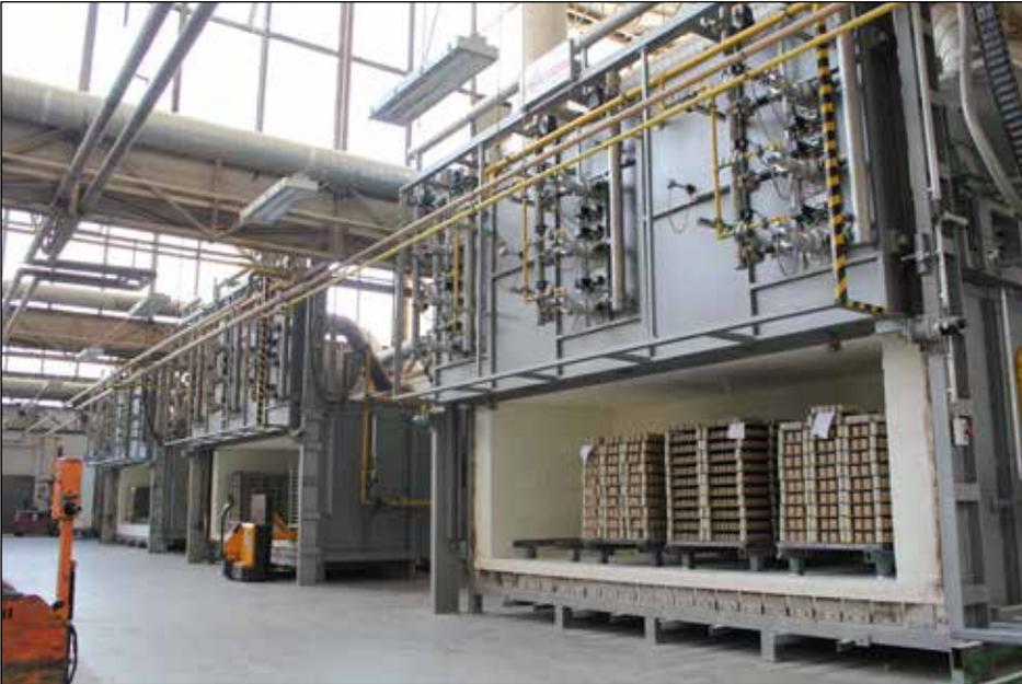
gas heated chamber furnace - 6m<sup>3</sup> - 1350°C
