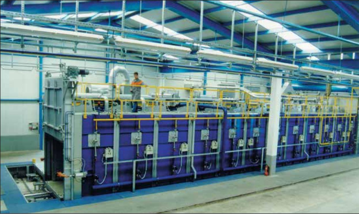
gas heated tunnel furnace - 12 x 28 m - 250°C
