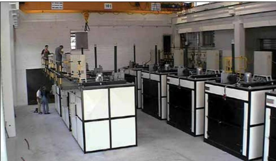
electro heated chamber dryers - 8m<sup>3</sup> - 250°C
