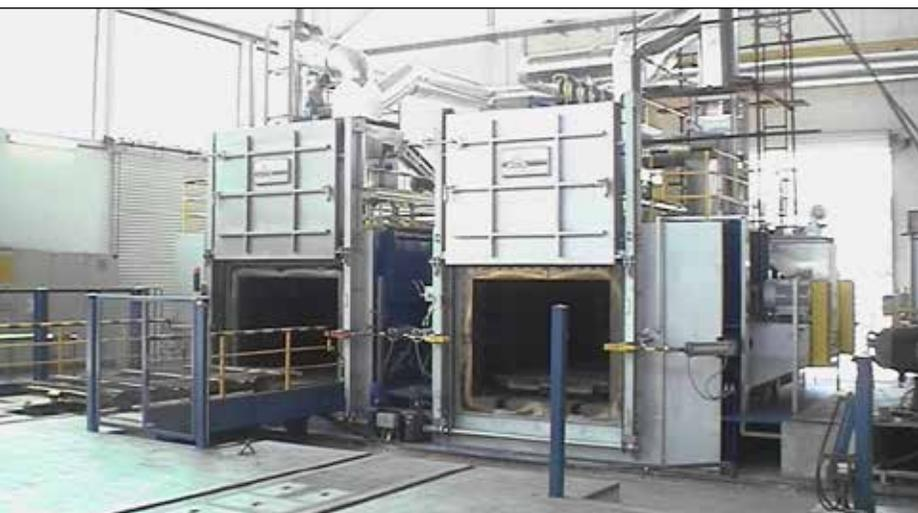
gas heated furnace - 5 tons - 550°C
