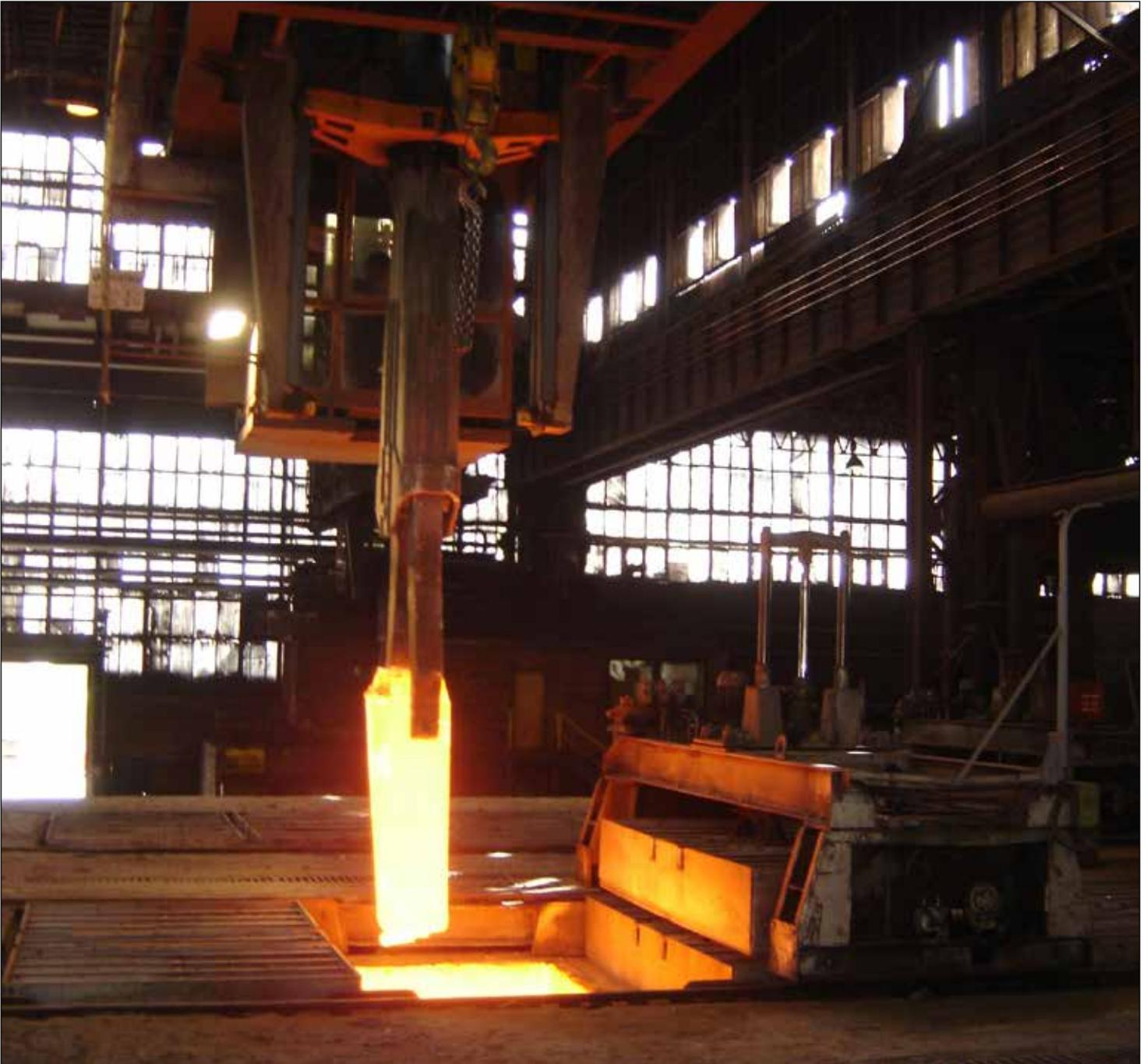
reheating gas heated furnace for ingots
