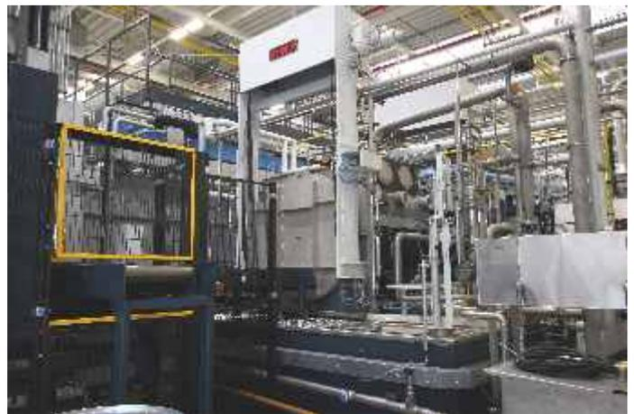
Fig.13 Flexiclean® continuous cleaning unit integrated into a pusher type gas carburizing plant
