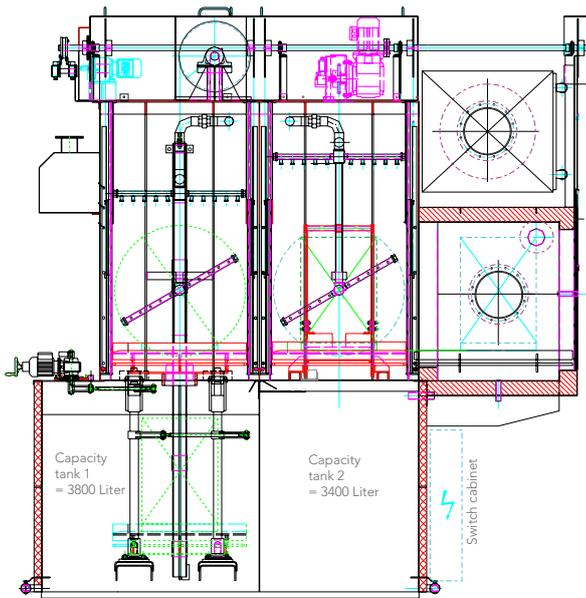
Fig.6 - Continuous submersion spray cleaning unit
