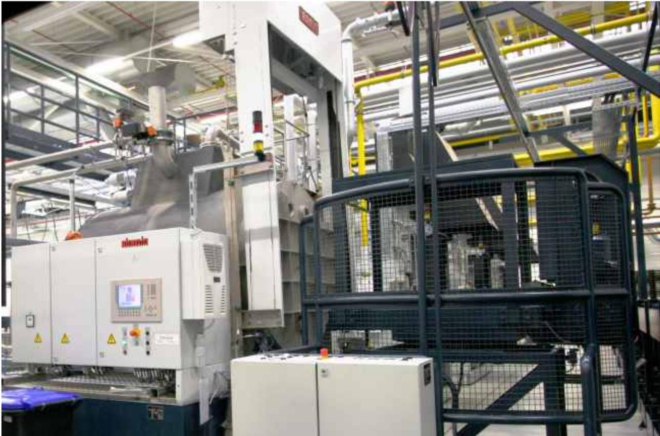
Flexiclean with 2 medium tanks integrated into a chamber furnace line
