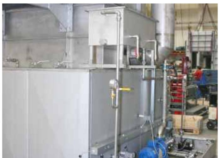
Fig.9 - Rear view chamber submersion spray cleaning unit with coalescence oil separator
