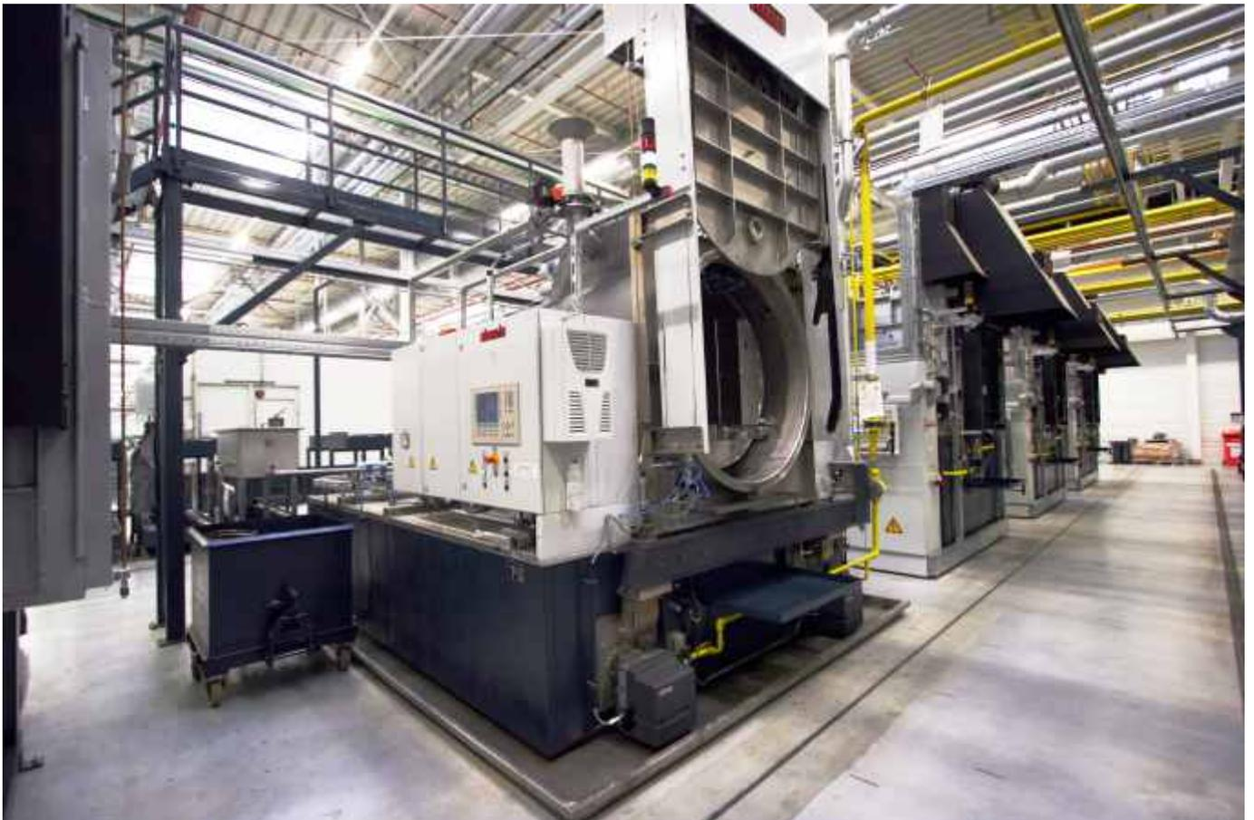
Fig.14 - Flexiclean® integrated in a double-chamber furnace line
