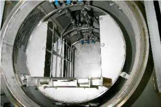
Fig.10 - Charge room Flexiclean® - chamber unit
