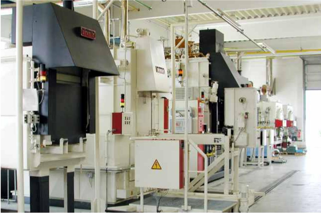
Chamber submersion spray unit integrated into a chamber furnace line
