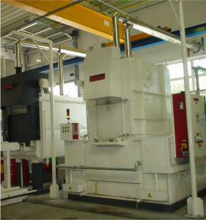
Fig.4 - Chamber submersion spray unit integrated into a chamber furnace line
