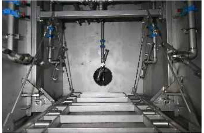
Fig.5 - Charge room chamber submersion spray unit
