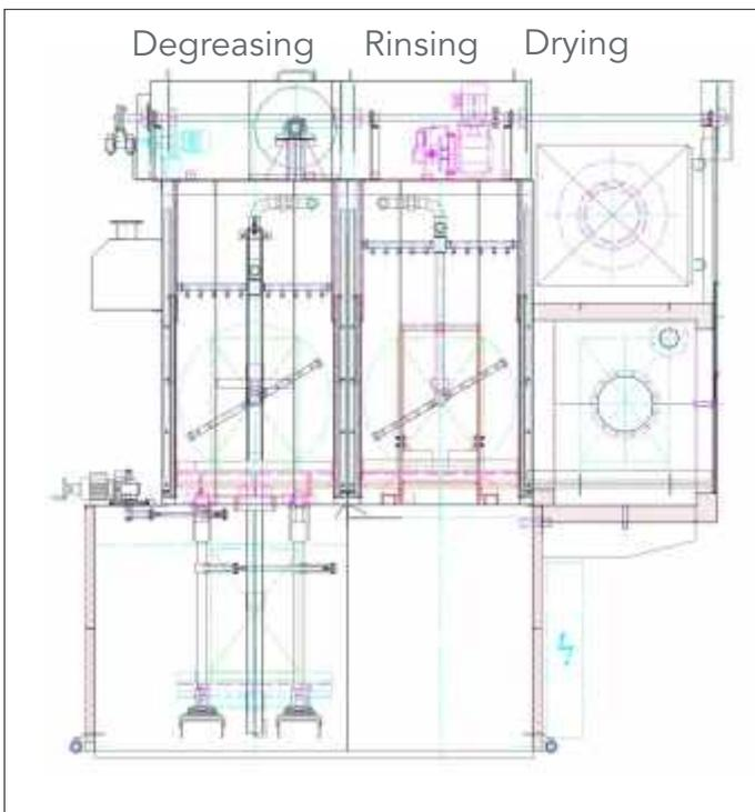
A rotary spraying nozzle system provides better cleaning quality.
