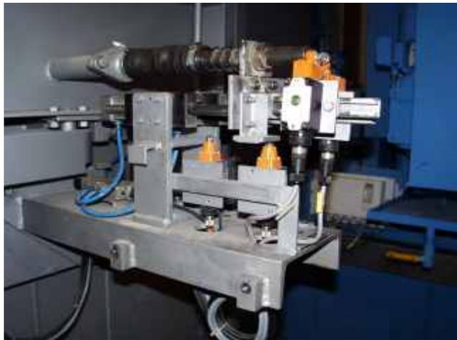
redirection of the trays with pusher and transversal pusher, are implemented in turnable way and can be adjusted in the setting operation with opened assembly door. This permits a precise and fast identification of the final position of the trays during assembling and putting into operation phase.
