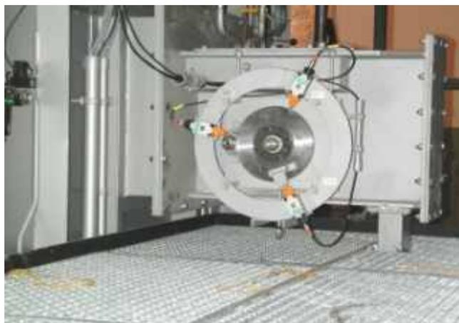
The transversal pusher is designed according to the lantern pinion principle, whereby a safe operability is ensured also with thermal expansions of the pusher chain.
